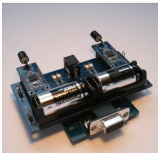
Gateways and repeaters use standard NTMs with function 2 (Repeater) activated.
